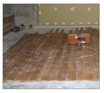
A test floor and 'tapping machine' at the CSIRO acoustic test laboratory in Melbourne
